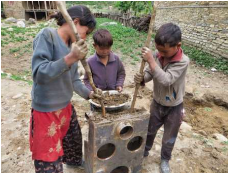
PIC.25. Children of a Pere family are filling mud into their new SMS.
