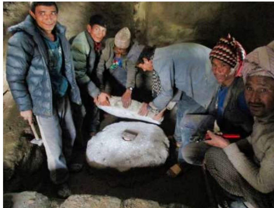
PIC.50. Pere men are installing the newly manufactured IWM milling stones.
